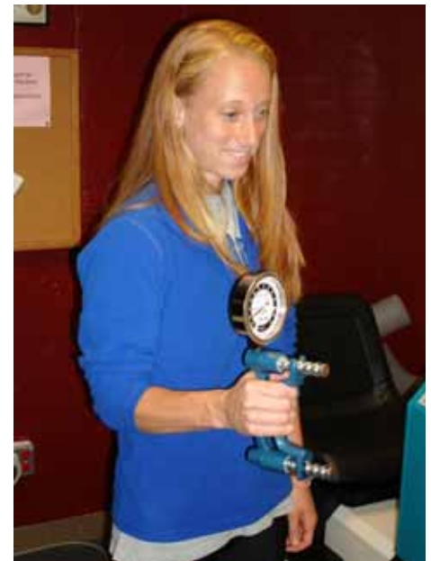
Figure 1. Grip strength is almost exclusively tested isometrically with a hand-held dynamometer.
